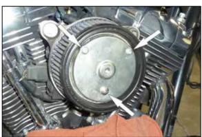
3. Remove the remove the three Torx screws that attach the air filter.
