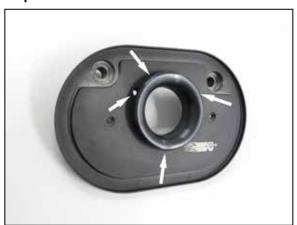
7. Install the provided intake velocity stack and the three throttle body bolts in the K&N® back plate.
