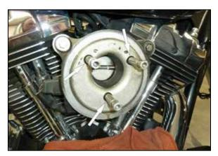
4. Remove the three back plate retaining bolts shown.
