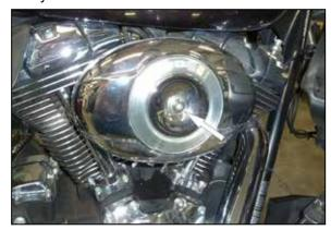
2. Remove the Allen screw that attaches the air
