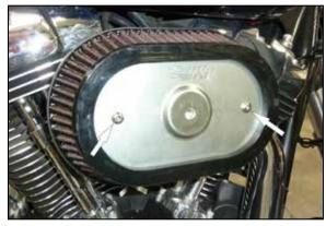
11. Place the K&N® filter on the back plate and attach with the remaining button head screws. NOTE: Apply one drop of provided thread locker to each screw.
